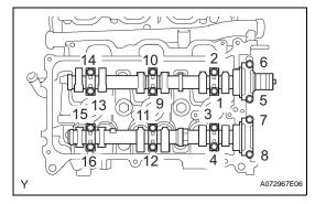
(f) Using several steps, uniformly install and tighten the 16 bearing cap bolts in the sequence shown in the illustration.
