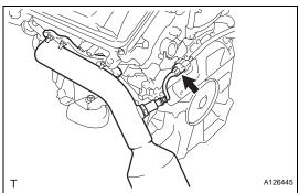
(c) Connect the air fuel ratio sensor connector.
