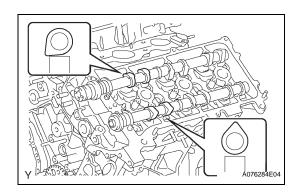
(c) Place the 2 camshafts onto the cylinder head with the cam lobes of No. 1 cylinder facing in the directions shown in the illustration.
