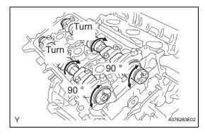
(g) Turn the camshafts clockwise until the knock pin comes to a position 90° to the cylinder head.
