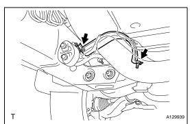
(c) Install the No. 2 front exhaust pipe with the 2 new nuts and 2 bolts.
