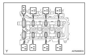
(d) Install the 8 bearing caps in the proper locations as shown.
