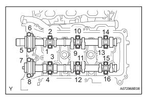
(f) Using several steps, uniformly install and tighten the 16 bearing cap bolts in the sequence shown in the illustration.
