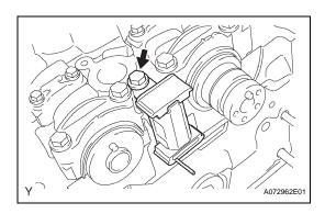
(b) Install the No. 2 chain tensioner with the bolt. Torque: 19 N\*m (194 kgf\*cm, 14 ft.\*lbf)
