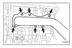
(b) Install the exhaust manifold with the 6 nuts. Torque: 30 N\*m (306 kgf\*cm, 22 ft.\*lbf)
