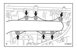
(b) Install the exhaust manifold with the 6 nuts. Torque: 30 N\*m (306 kgf\*cm, 22 ft.\*lbf)
