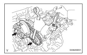
(d) Hold the hexagonal portion of the camshaft with a wrench, and tighten the 2 bolts.
